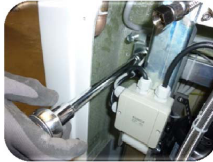
Picture 8: Loosen and remove the upper fastening screws (left).
