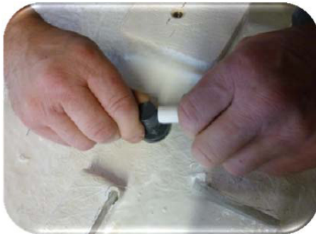
Picture 7: Pull the air hose off the connecting valve.
