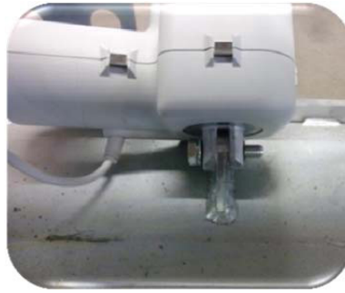
Picture 10: Remove the screw, incl. the washer, from the lower motor mount.
