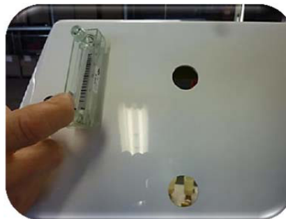
Picture 10: You can take the flow meter out of the control panel.
