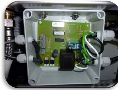
Picture 8: Guide the cable through the PG threaded connection into the distributor unit and clamp the cable of the sensor. Then screw on PG threaded connection again.
