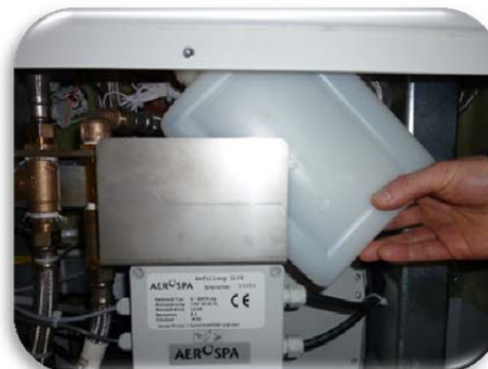
Picture 4: Take out the disinfectant container by pulling it diagonally out of the bracket.
