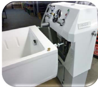
Picture 15: Take the tub body out of the lifting frame.
