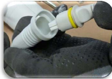
Picture 11: Remove the connecting cable from the lifting motor.
