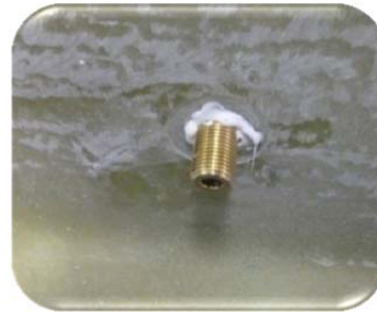
Picture 14: The illustration shows the connecting valve removed from the air nozzle.
