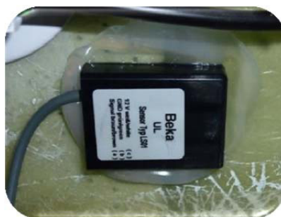
Picture 3: Loosen the sensor using a carpet knife.
