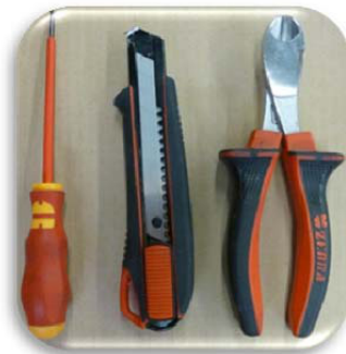
Picture 1: Required tools: 1 x slotted screw driver, small 1 x carpet knife 1 x combination pliers
