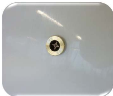
Picture 11: The illustration shows the cover removed from the air nozzle.
