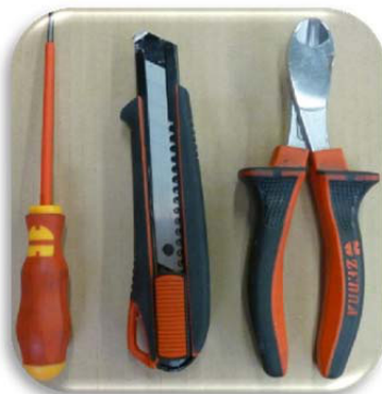
Picture 1: Required tools: 1 x slotted screw driver, small 1 x carpet knife 1 x combination pliers
