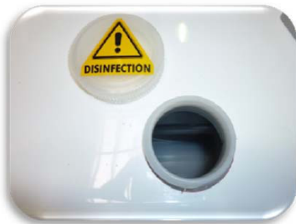
Picture 3: Remove the threaded connection from the disinfectant container.
