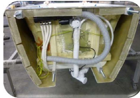
Picture 16: The illustration shows the tub body removed from the lifting frame.
