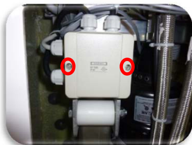
Picture 3: Open the distributor unit and unclamp the line for the fan motor.
