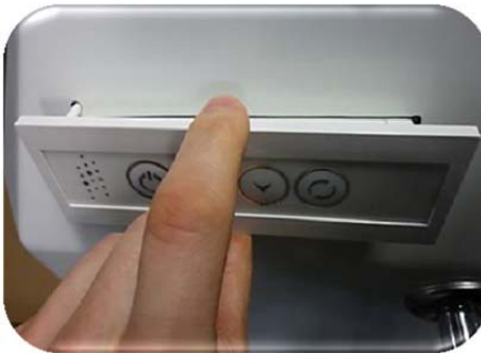
Picture 9: The illustration shows the removal of the operating element.
