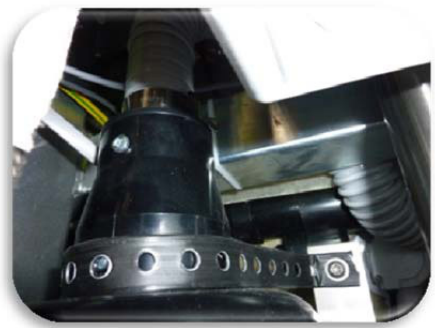
Picture 13: Loosen the hose clamp on the fan motor and take out the hose.
