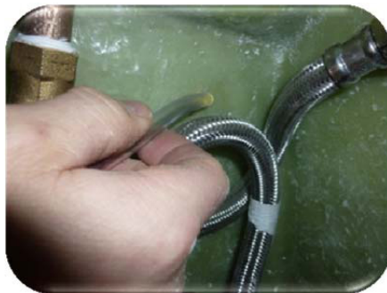
Picture 9: Remove the 2 fastening clips from the flow meter.
