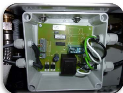
Picture 5: Unclamp the cable from the sensor and take the cable out of the distributor unit. Note that the PG threaded connection must be opened.
