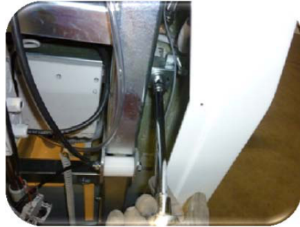
Picture 7: Loosen and remove the upper fastening screws (right).
