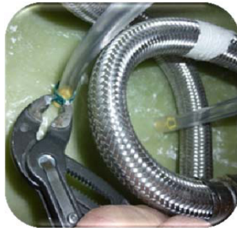
Picture 5: Remove the hose clamps from behind.
