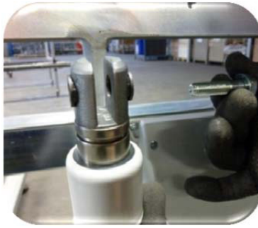
Picture 9: Remove the screw, incl. the washer, from the upper motor mount.
