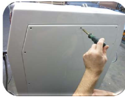
Picture 2: Remove all screws (9 pcs.) from the rear wall.
