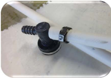
Picture 5: Disconnect the hose clamp from the hose.
