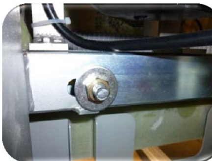
Picture 10: Loosen and remove the upper fastening screws (left and right).
