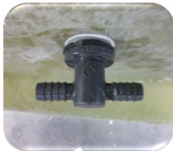
Picture 9: The illustration shows the connecting valve screwed on.
