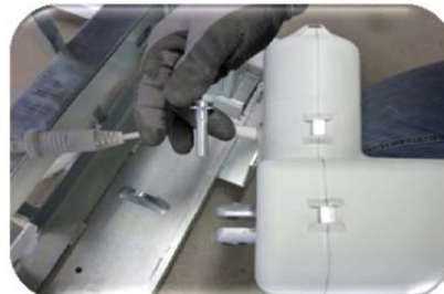
Picture 12: Remove the screw from the lower motor mount and take the lifting motor out of the lifting frame.
