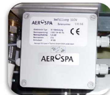
Picture 4: Open the distributor unit in order to unclamp the cable from the sensor.
