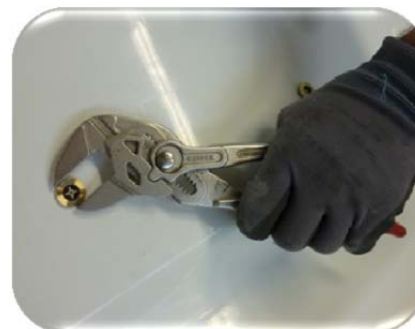
Picture 12: Hold the air nozzle tightly from above using pliers with no teeth.
